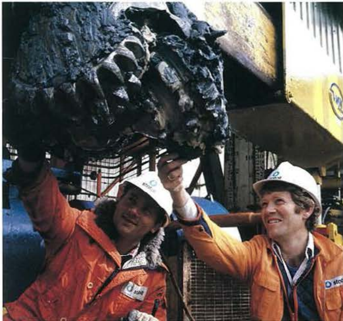
The first drill bit is a hole opener with a diameter of 36 inches.
