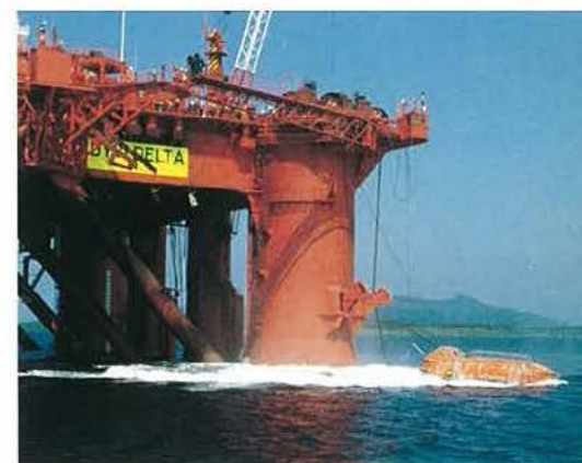
The free-fall lifeboat is tested. The Dyvi Delta, which is drilling for Statoil, is the world's first drilling rig with this emergency system.
