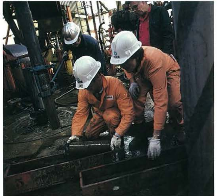
Rock samples, so-called core samples, are taken in interesting zones.
