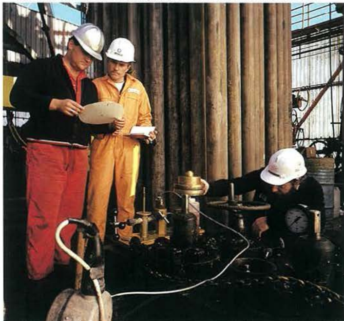
Continuous measurements on oil and gas properties are taken when a well is tested for production.
