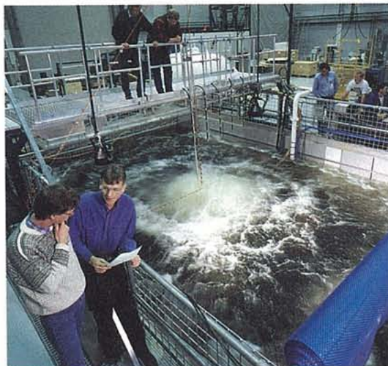
Experiments with gas emissions under water are being pursued in the test tank at Statoil's Research Centre in Trondheim.
