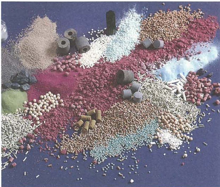
CATALYSTS: A catalyst promotes a chemical reaction. Such substances play a crucial role in processing oil or gas. Key research targets for Statoil include boosting the production rate of a principal product and reducing unwanted by-products.
