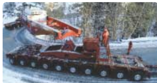
A technically advanced, though massive trailer, climbing steep winter roads to Liertoppen and Sylling transformer station in Southern Norway. The transformer payload in question gave this equipment a combined weight of 400 tons. Safety is an absolute condition.
