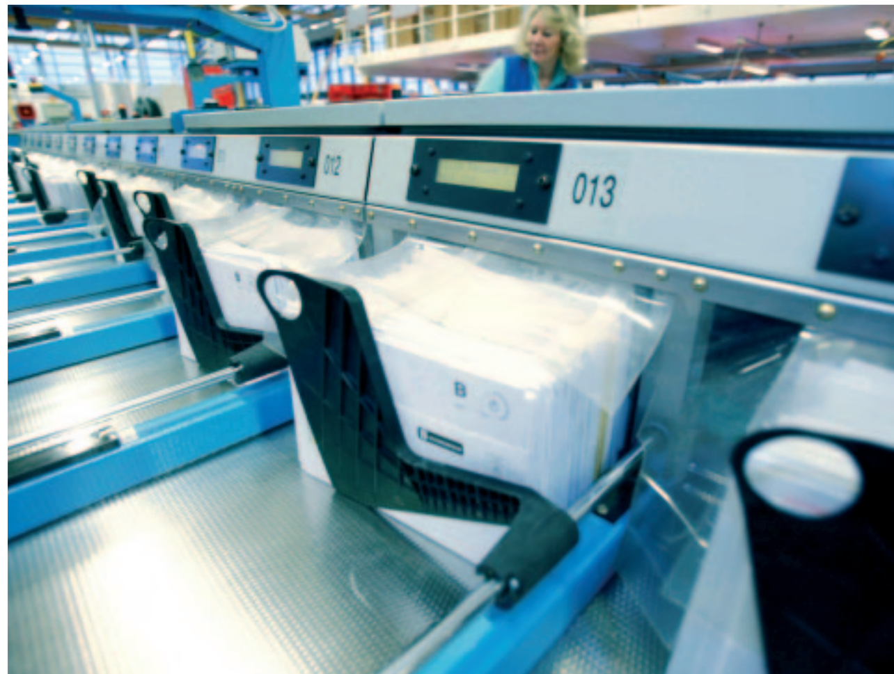
Delivers: One person can sort about 1 400 letters an hour, whereas a machine can handle some 27 000 letters during the same time. This photo is taken at the terminal at Stokke, Vestfold county.
