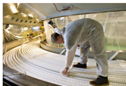
Impregnation of the NorNed cable at the Nexans factory in Halden
