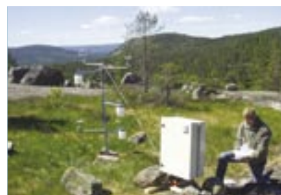
NILU technician Tore Hansen installs an instrument for measuring dry deposition of reactive nitrogen compounds in Telemark, Norway.
