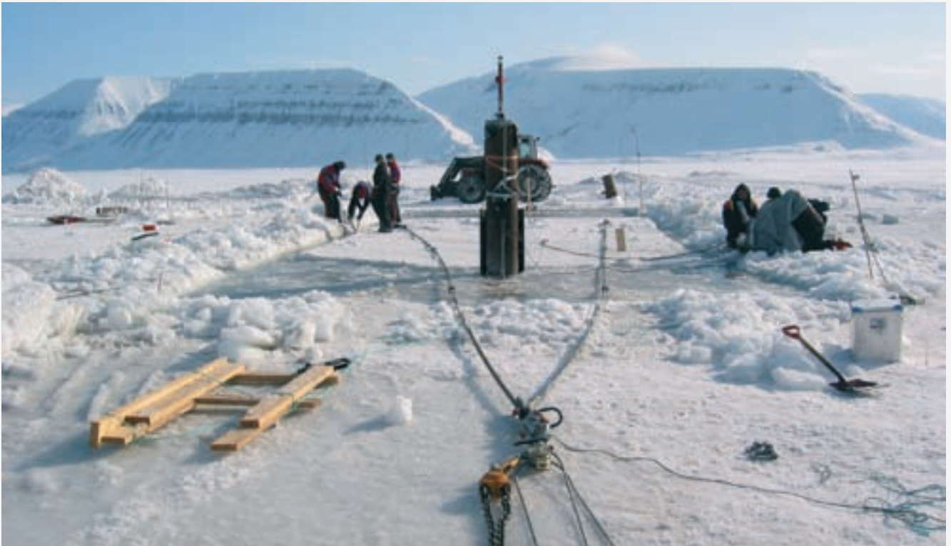
Arctic Technology has been doing medium scale ice-structure interaction experiments on the sea ice in the Van Mijen fjord. An ice floe was towed so that it crushed against a pile while forces and displacements were measured. Photo: Lars Grande
