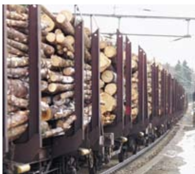
A timber train can carry as much as 20 articulated trucks. Photo: Sven Goll
