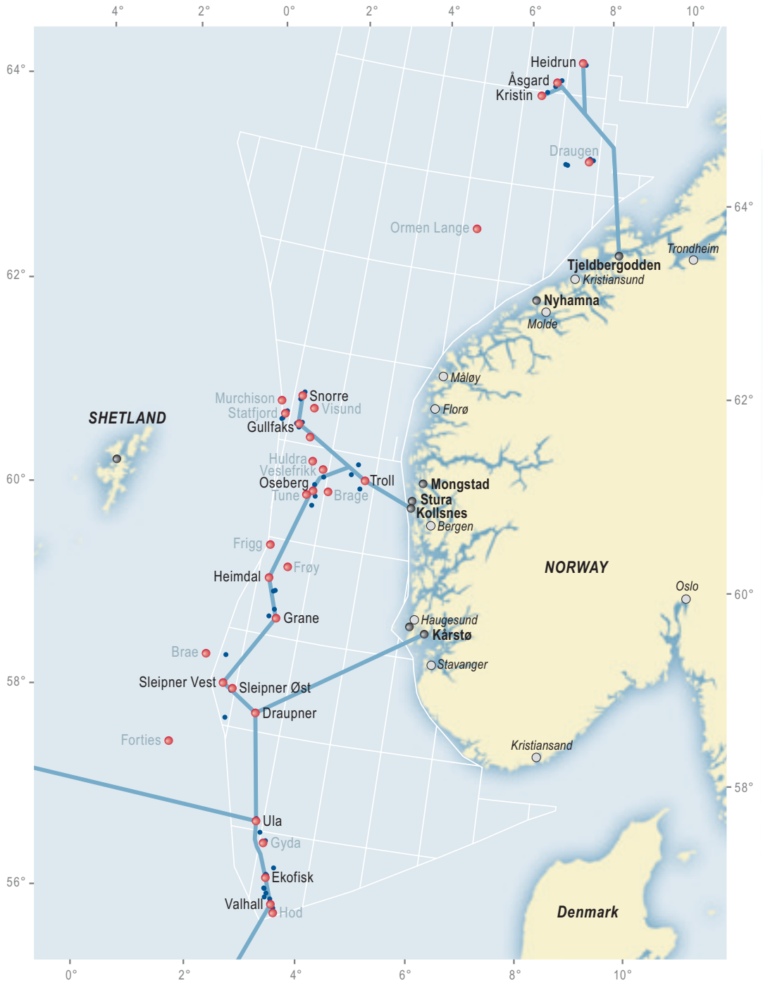
Figure 4.5 Optical fiber cables on the Norwegian continental shelf (Source: Norwegian Petroleum Directorate)
