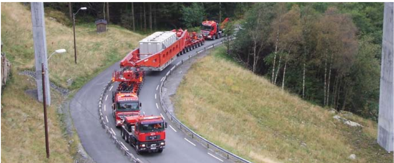
Eight transformers have been produced for the NorNed project, four for each country, and each weighing about 250 tonnes.
