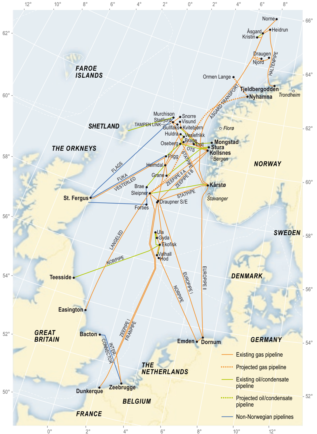
Figur 14.1 Existing and projected pipelines (Source: Norwegian Petroleum Directorate)
