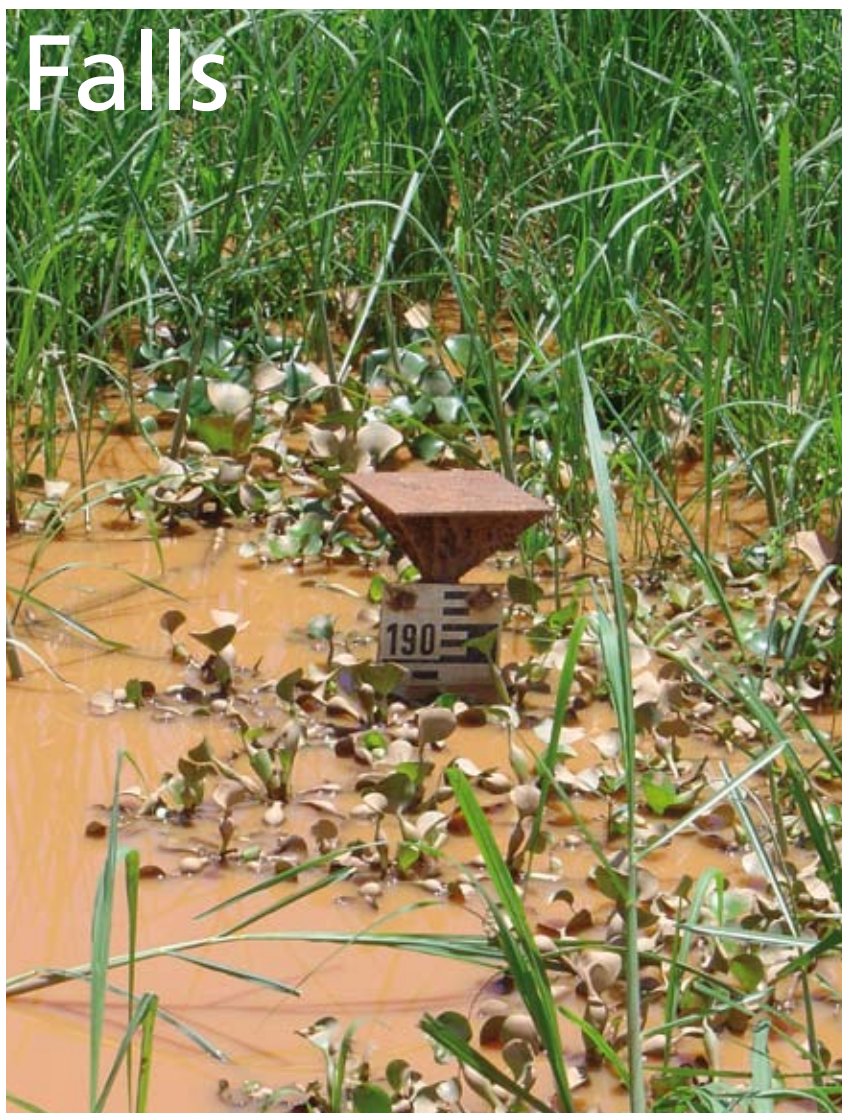
Operational staff gauge upstream of Rusumo Falls
