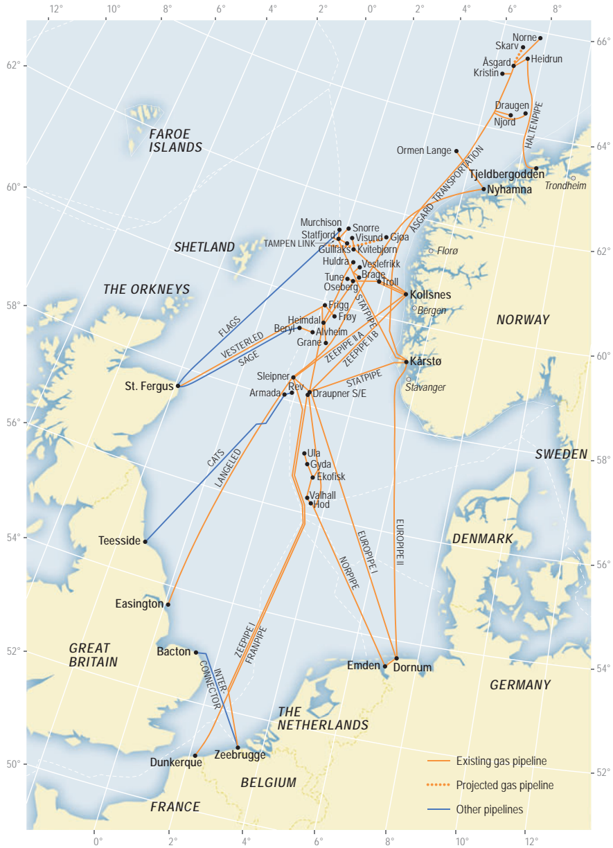
Figure 6.1 Gas pipelines (Source: Norwegian Petroleum Directorate)
