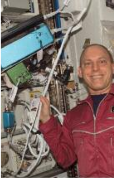
The ANITA trace gas monitor, developed mostly by SINTEF, was tested on the Space Station. The test results were so promising that ANITA may be permanently installed in the Space Station and in other space vehicles. ©NASA
