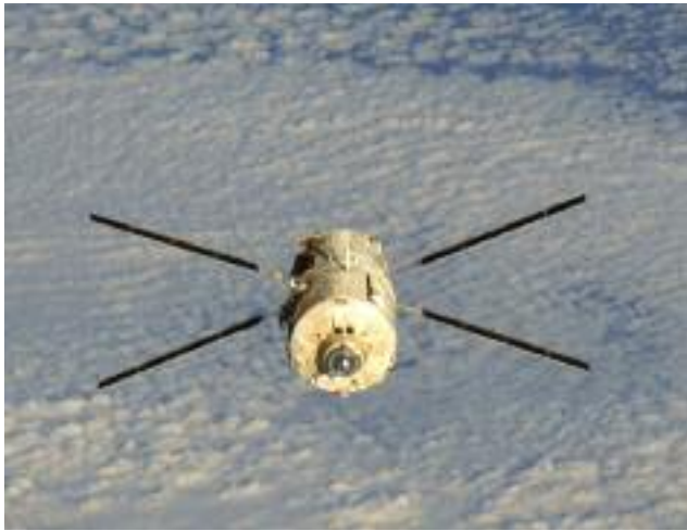
The Jules Verne Automated Transfer Vehicle (ATV), a resupply spacecraft, was launched from French Guiana on a trajectory for the International Space Station. It arrived in April and automatically docked with the Space Station, to resupply it with air, water, food, equipment and clothing for the astronauts in space. ©NASA
