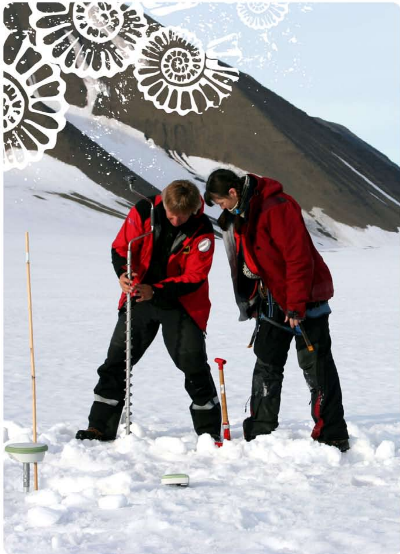
August 2008: Pilot Bjørn F. Amundsen helps Ph.D. student Monica Sund drill through the thick snow layer on top of Kroppbreen. Kroppbreen is in a partial surge stage and Sund's project aims at monitoring the surge from start to finish.
