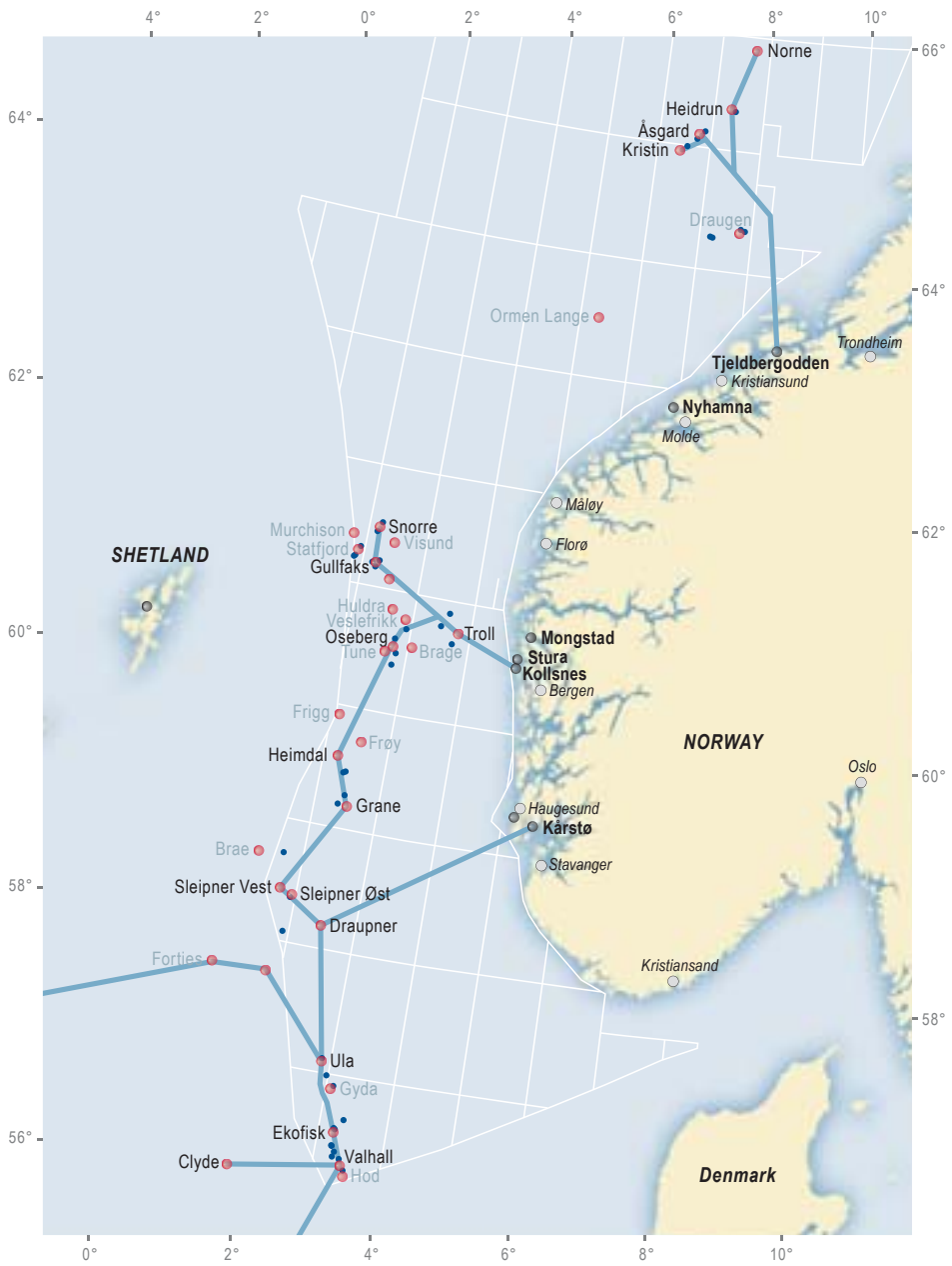
Figure 5.6 Fibre-optic cable network on the Norwegian continental shelf (Source: Norwegian Petroleum Directorate)
