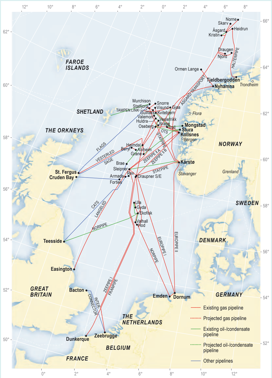
Figure 14.1 Existing and projected pipelines (Source: The Norwegian Petroleum Directorate)
