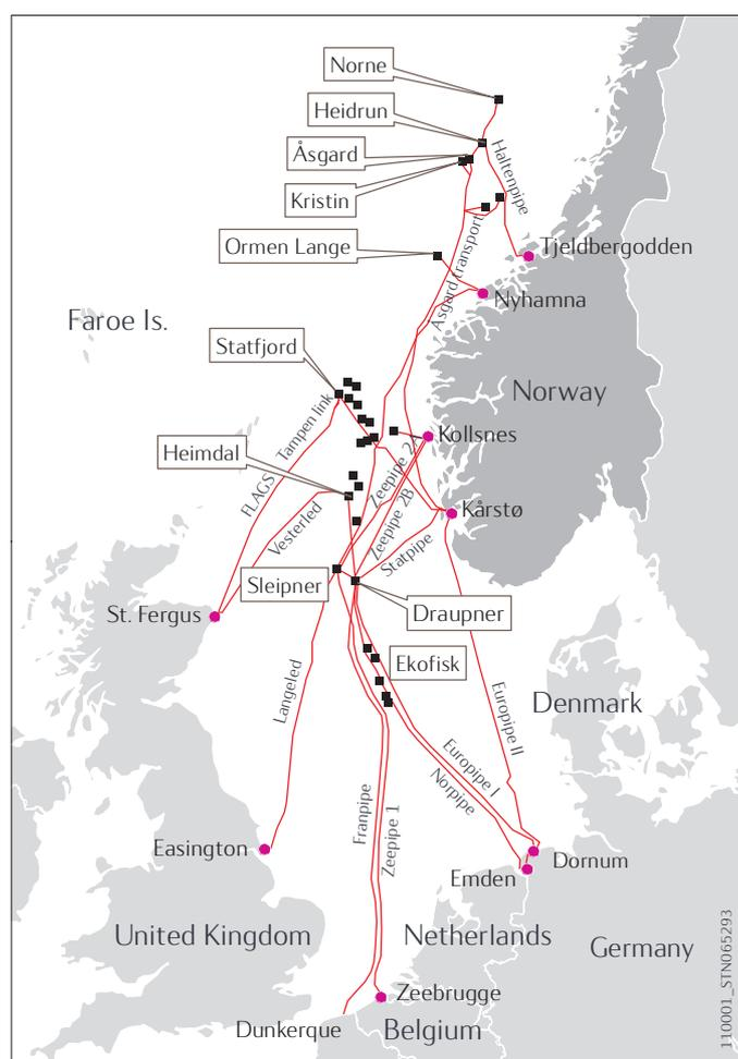
The total length of Norway's gas pipelines is currently 8,100 kilometres. All gas pipelines on the NCS with third-party customers are owned by a single joint venture, Gassled, with regulated third-party access. The Gassled system is operated by the independent system operator Gassco AS, a company wholly owned by the Norwegian state. In 2011, the Gassled system transported 94.2 bcm (3.3 tcf) of gas to Europe.
