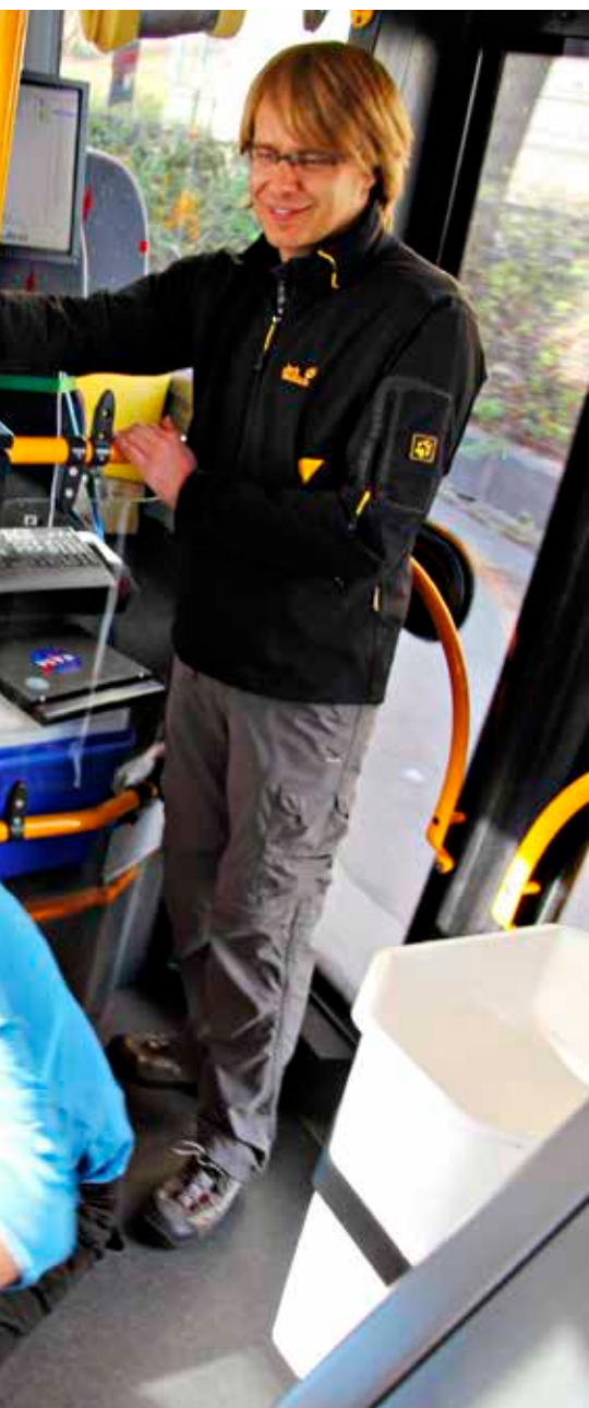
Armin Wisthaler (right) and Tomas Nikovini measure the exhaust from an ethanol bus using the PTR instrument. Photo: Lone Lohne, Aftenposten
