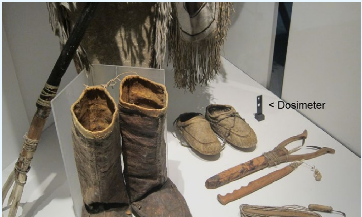
The dosimeter is a small holder for two tiny pieces of glass, which reacts with pollutants in the air. Here it is in a display case in the Museum of Cultural History in Oslo. Photo: Anne Sommer-Larsen, Museum of Cultural History.
