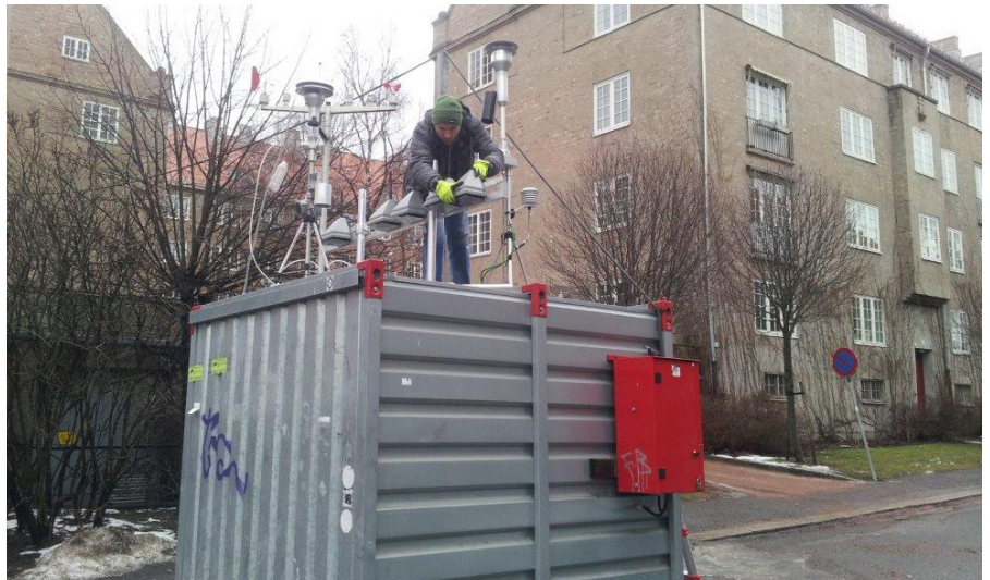
Scientists from NILU and the Technion Israel Institute of Technology evaluated 24 low cost AQMESH sensors (below) in 2015. These sensors were mounted on top of the traffic oriented monitoring station in Kirkeveien (above), so that the scientists could compare measurements from the AQMesh sensors to air quality measurements from the monitoring station at the same location.
