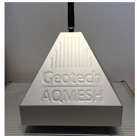
Scientists from NILU and the Technion Israel Institute of Technology evaluated 24 low cost AQMESH sensors (below) in 2015. These sensors were mounted on top of the traffic oriented monitoring station in Kirkeveien (above), so that the scientists could compare measurements from the AQMesh sensors to air quality measurements from the monitoring station at the same location.
