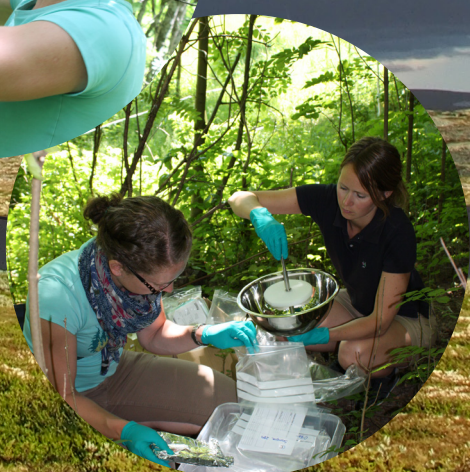
The scientists putting together a UFO at Bærums Verk. The disc in the middle is the filter that captures various environmental contaminants from the air.
