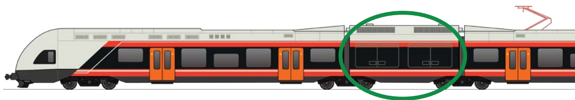
The bimodal Flirt train is actually a completely ordinary electric train set. The only difference is that it has a short wagon where diesel engines are located. These act as generators and supply power to the train's electric engines. Source: Infokraft/Jernbanemagasinet
