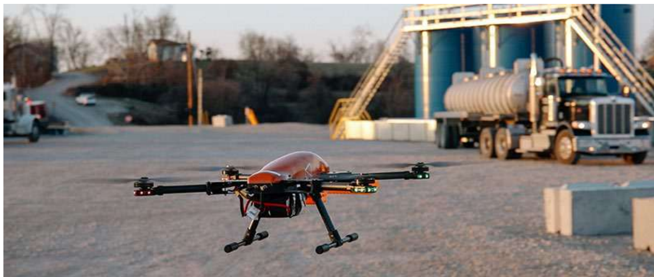
Drone technology (SeekOps) being used in methane detection, Appalachian basin in Ohio, USA.
