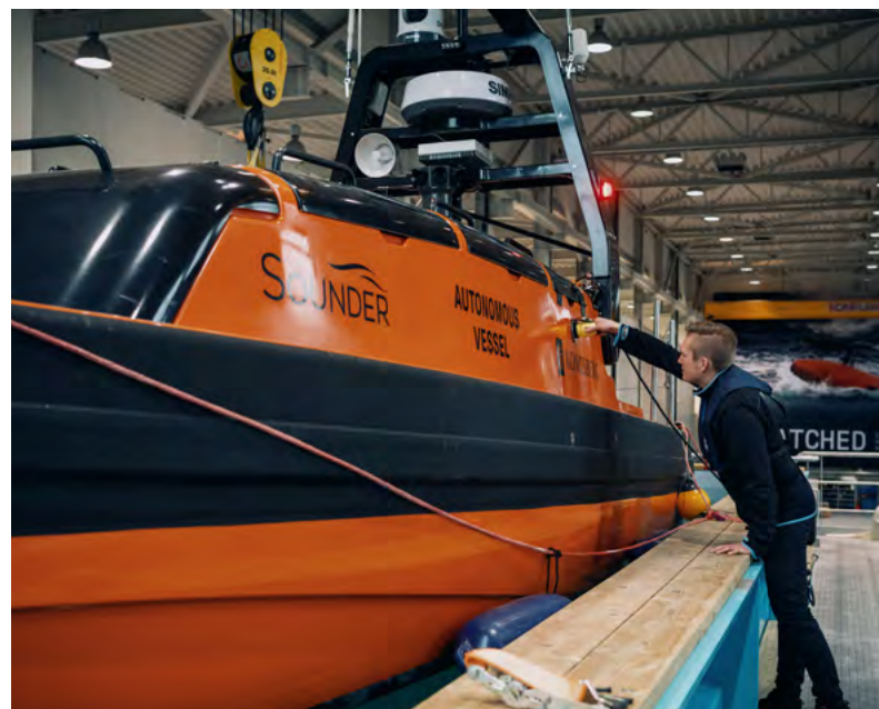
◀ The award-winning Sounder USV is a multi-purpose unmanned surface vehicle system with a unique hull design to ensure high performance for hydroacoustic applications. Here photographed at our site in Horten, Norway. This is one of the key products delivered by Sensors & Robotics, a division of Kongsberg Maritime in 2022, but as of 1 January 2023 reports a separate business area of the Group.
