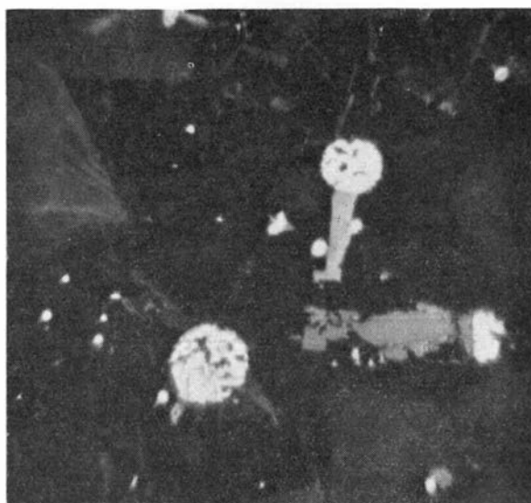
Fig. 2. Polished section showing globules and globular aggregates of pyrite (white) and ilmenite (grey) in a base of devitrified glass (black), showing minute, elongated crystals of unidentifiable minerals. Ordinary light.
