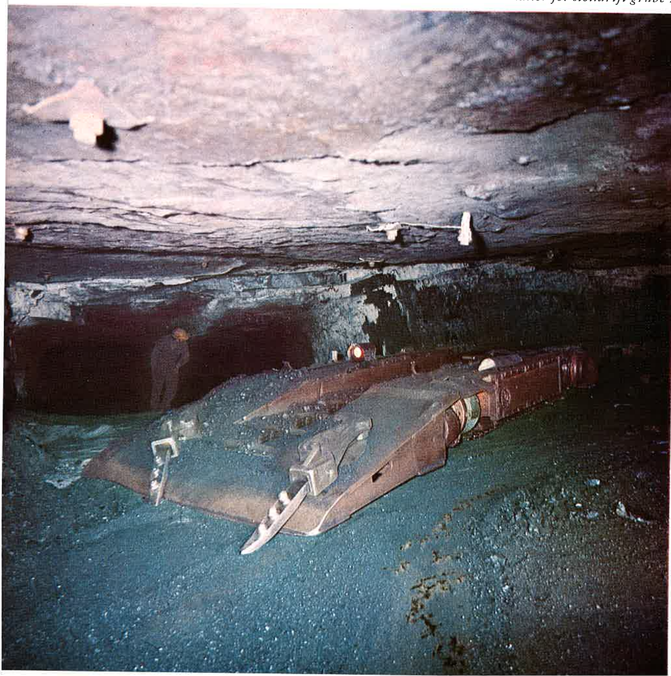
Maskinlaster for stollrift grube 7
