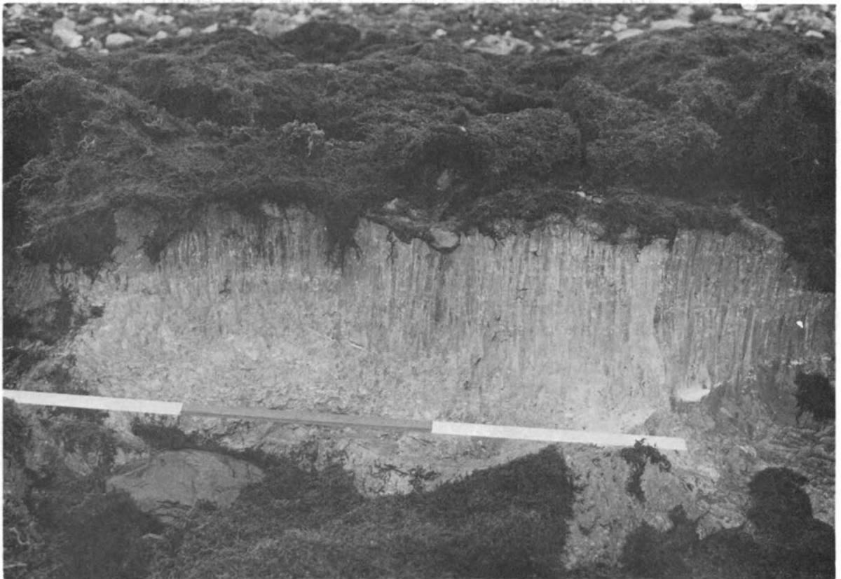
Fig. 4. Vertically orientated crystals with the overlying moss cover. The scale is marked in feet (0.3 m).
