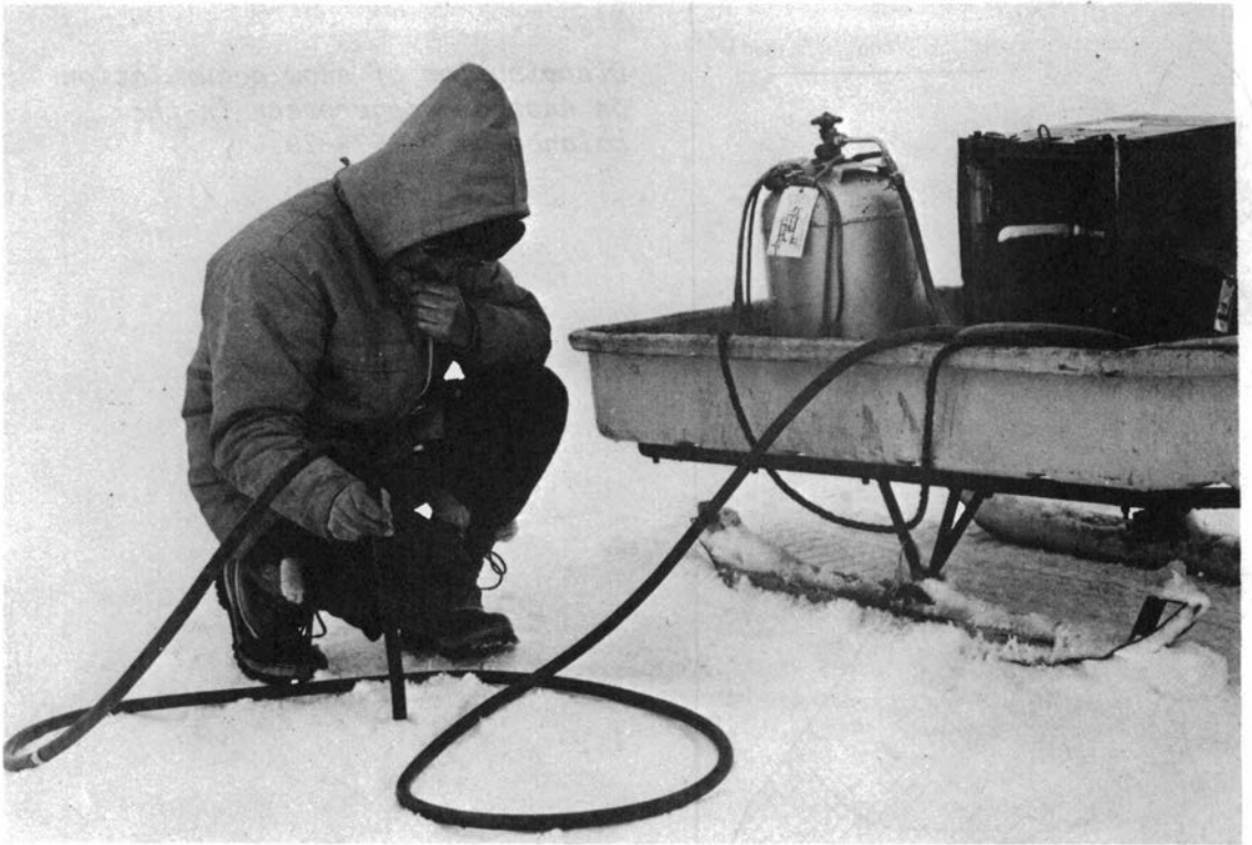
Fig. 5. Steam drilling at Brøggerbreen. The steam is generated in a pressure boiler and led through an insulated hose to a nozzle at the end of a metal rod. A 10 m deep vertical hole is drilled with a speed of about 20 cm/minute with this equipment.
