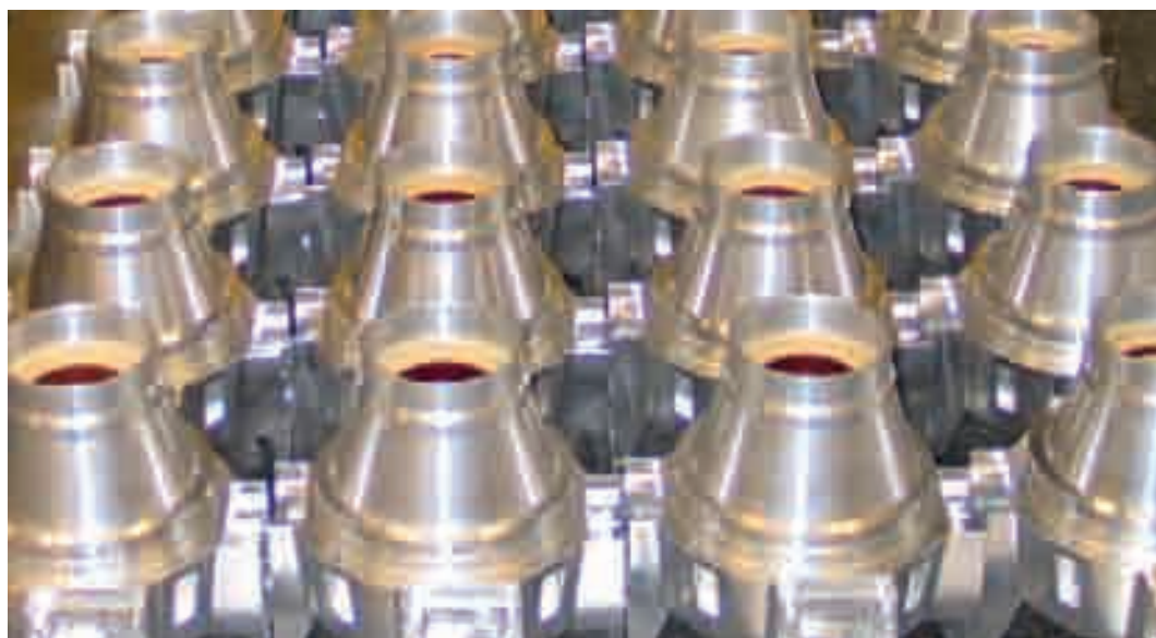
IRIS-T Exit Cones, in two operations these units are automatic measured for nearly 150 defined characteristics each.
