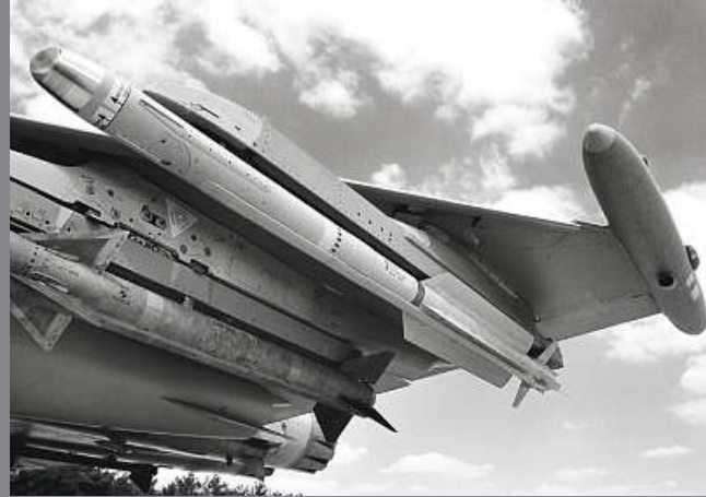
IRIS-T MISSILE ON EUROFIGHTER WITH ROCKET MOTOR FROM NAMMO PHOTO: NAMMO ARCHIVE
